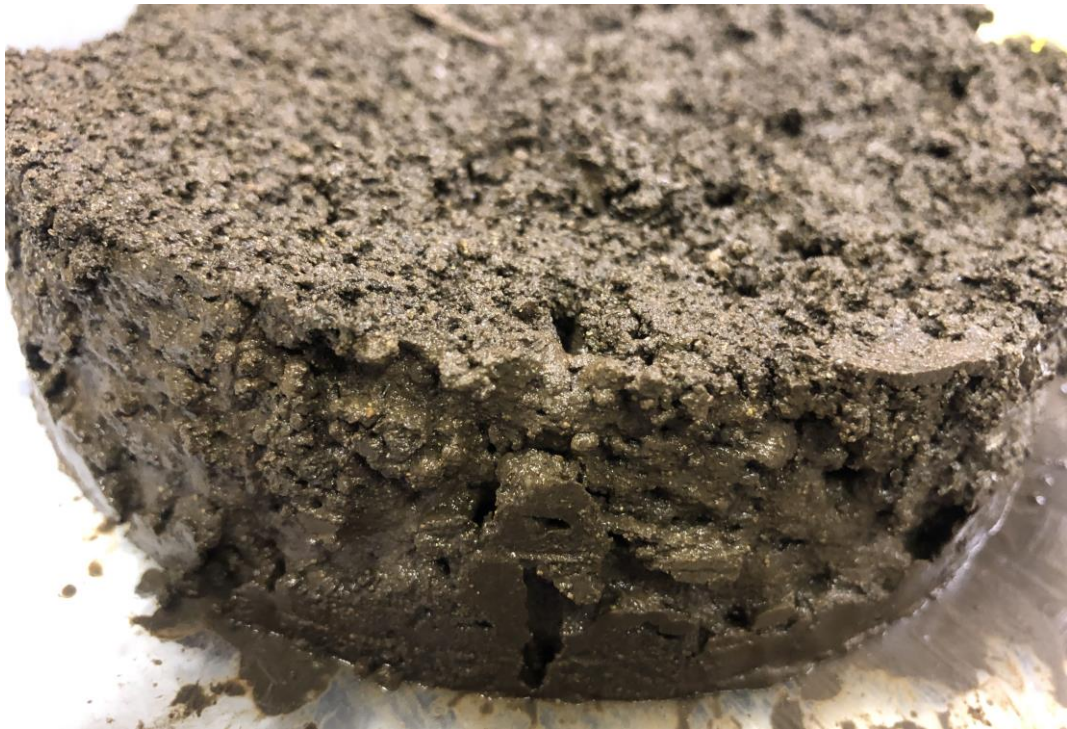
Photo. 3-9 Depth of EII ( 3 worms ) at 28 days for 4 ~ 8 cm column layer
