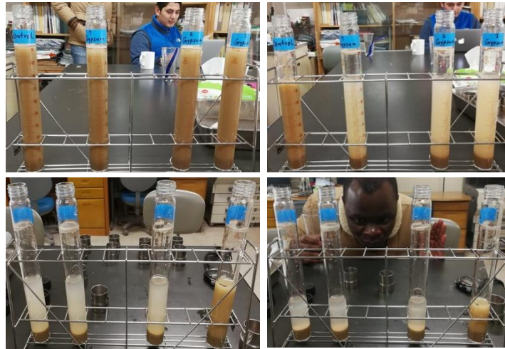
Fig. 4.23 Sedimentation as observed at 5 minutes interval
