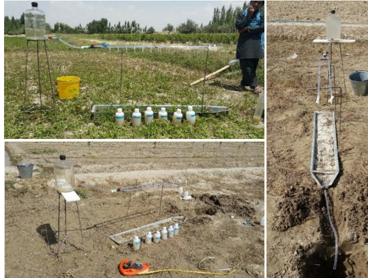
Fig. 4.5 Portable rainfall simulator and surface runoff collection
