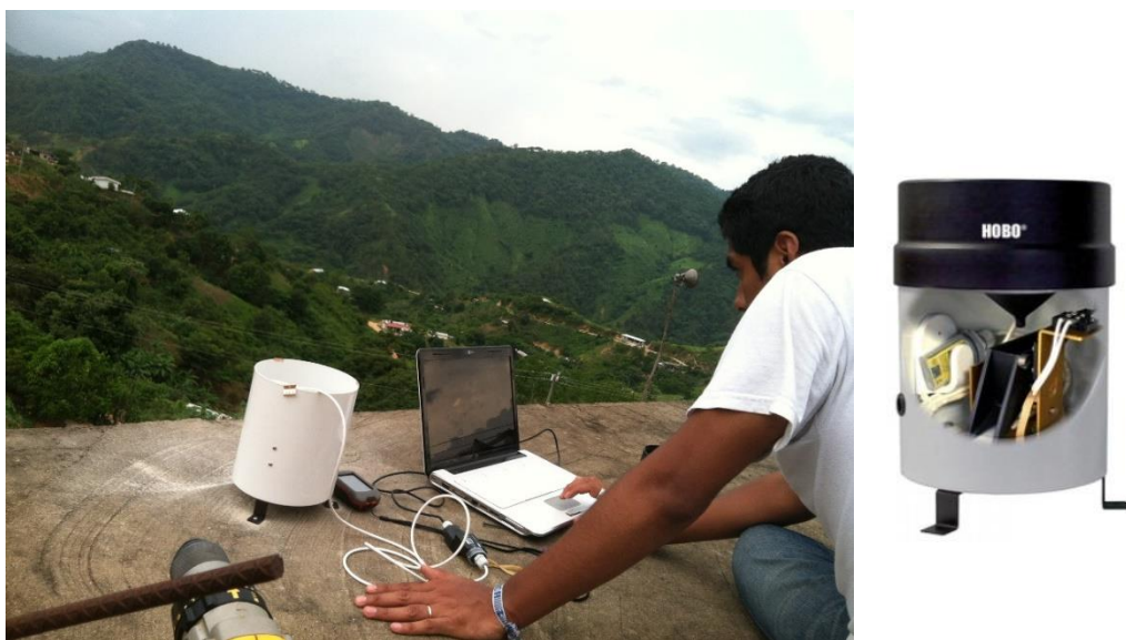
Fig. 2-8 Rain Gauge installed in El Jicaral Village
