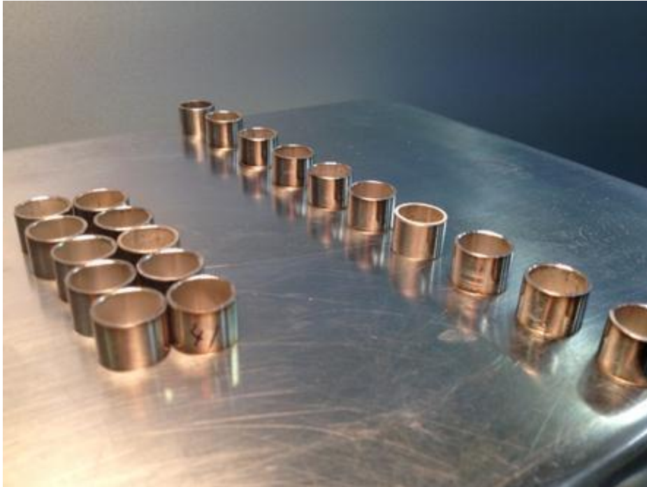
Fig. 4-4 Stainless cores for raindrop experiment
