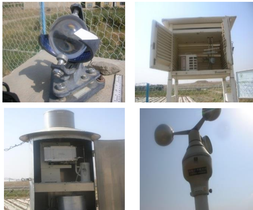
Fig. 3-5 (Upper-Left) Sunshine hour, (Upper-Right) Air temperature and relative humidity, (down-Left) Rain gage and. (Down -Left) Wind speed
