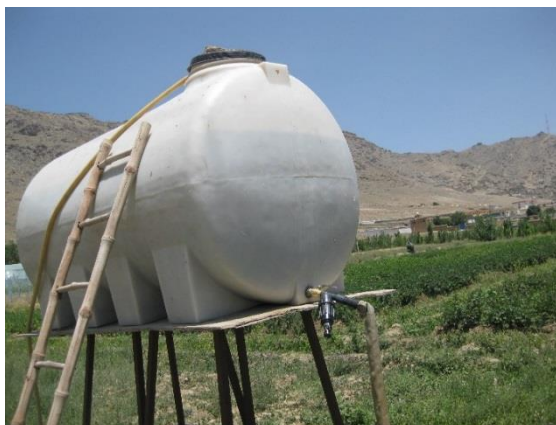
Fig. 5-11 water tank with filter connected to pipe
