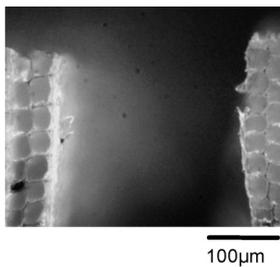
**Fig. 7** Separation of tracheids from rays in early wood.
