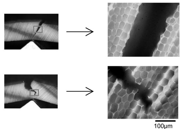
**Fig. 5** Crack propagation in radial direction.
