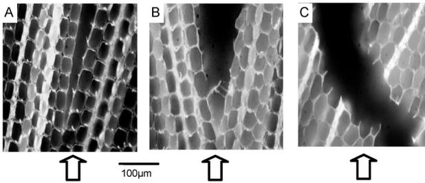
**Fig. 2** Typical patterns of crack propagation in early wood, **A**: separation between cells, **B**: partial splitting of a cell wall, **C**: rupture of a cell wall.
