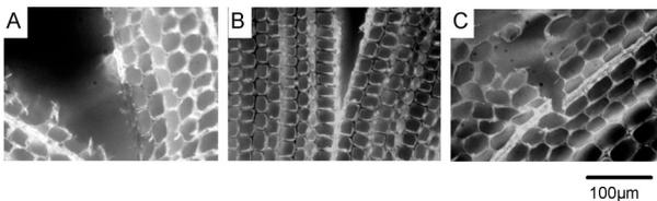
**Fig. 8** Crack propagation in rays.
