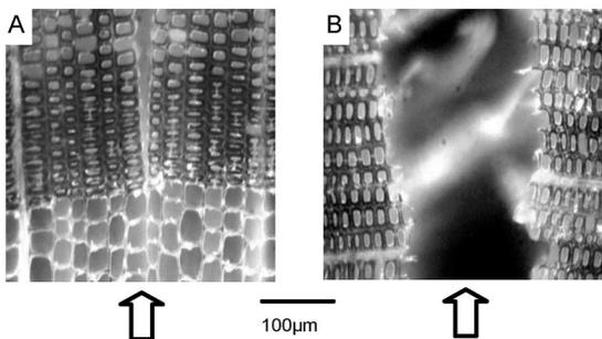
**Fig. 3** Typical patterns of crack propagation in late wood, **A**: separation between cells proceeded in the radial direction, **B**: splitting of cell wall in the tangential direction.
