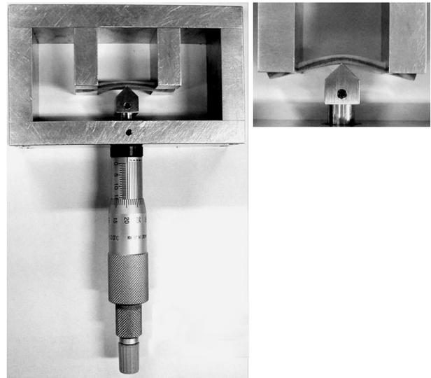
Fig. 1 Side view and a close up view of device for three-point bending test.
