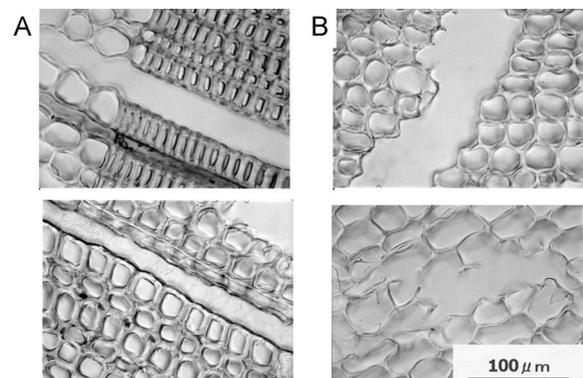
**Fig. 10** Modes of lathe checks progressed to radial (A) and tangential (B) directions.
