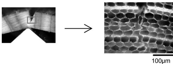
**Fig. 6** Crack propagation in radial direction.
