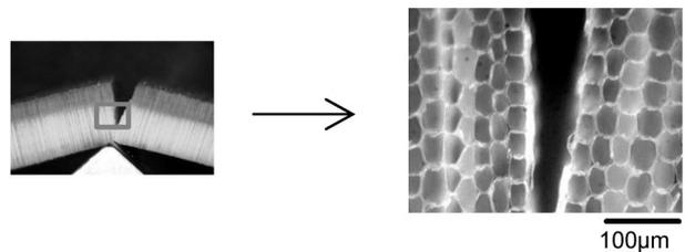
**Fig. 4** Crack propagation in radial direction.
