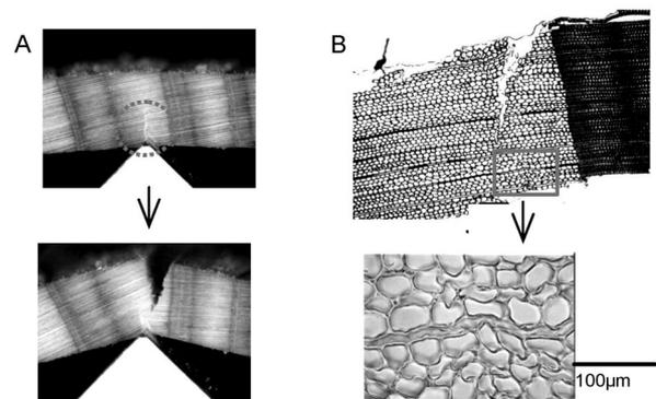
**Fig. 9** Comparison of crack propagation in bending (A), and a lathe checks in a chip (B).
