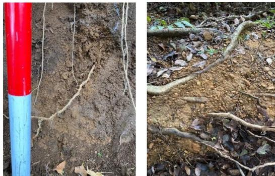
Figure 6. Soil profile of the survey area. The A layer was about 20 cm deep, and below that was clay soil.
