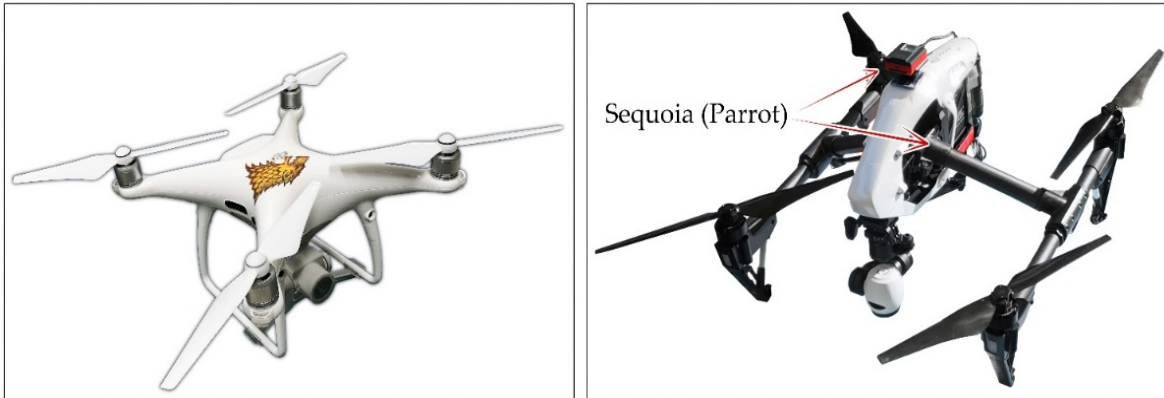
Figure 6.3. Unmanned aerial vehicles (UAVs) used for the aerial surveys: (a) Phantom 4 Pro (DJI); (b) Inspire 1 (DJI) with Sequoia (Parrot)
