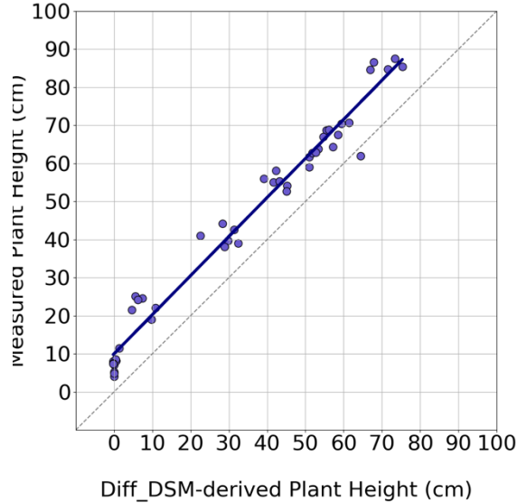
Figure 3.5 (b) Relationship between the estimated plant height by DSM and measured plant height of Potato
