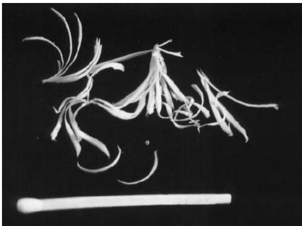
Fig. 2 Spiral chips produced by our chipping Machine
